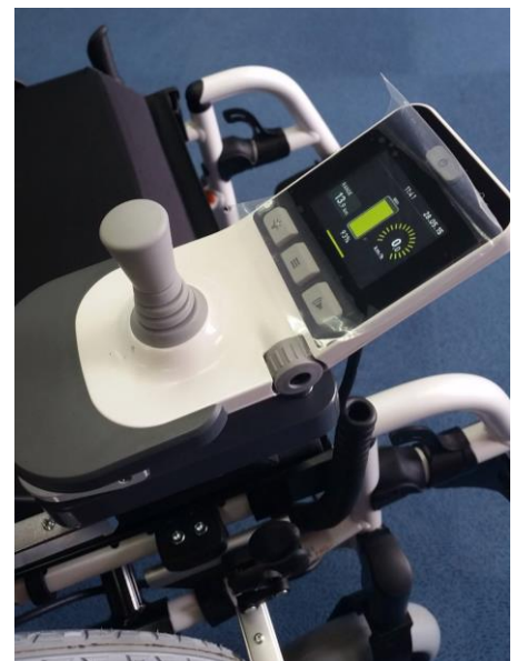
The E-Fix control pod and joystick
