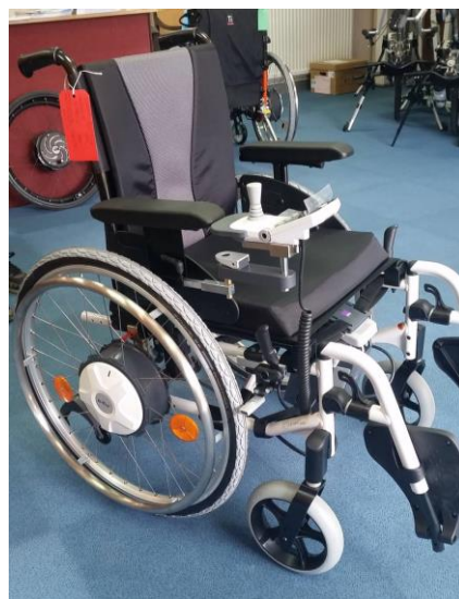
The Alber E-Fix components attached to a manual wheelchair.
